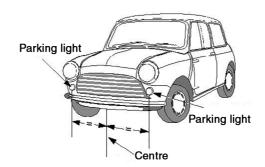
*Example of the position of a pair of parking lights fitted to a motor vehicle with 4 wheels—*
