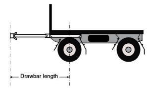
(2) For a trailer with 1 axle group or a single axle, other than a semitrailer, the distance between the pivot point of the coupling on a drawbar of the trailer and the centre line of the trailer's axle group or single axle must not be more than 8.5m.
