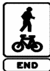
End shared path sign
