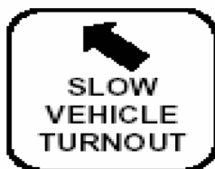
Slow vehicle turn out lane sign
