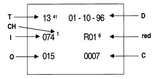
T is the time, in 24-hour clock mode, when the image was captured.
