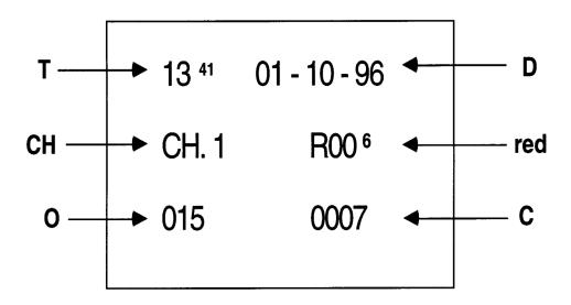
T is the time, in 24-hour clock mode, when the image was captured.
