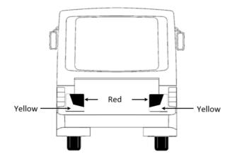
Example of an alternative patter for rear marking plates—
