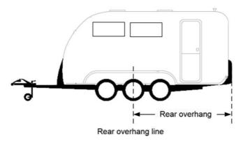
Example of the rear overhang and rear overhang line for a semitrailer—
