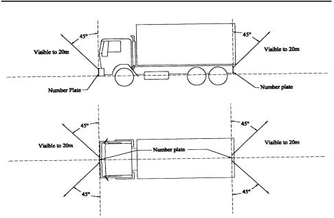
Figure 1—vehicle to which subsection (1)(a) applies
