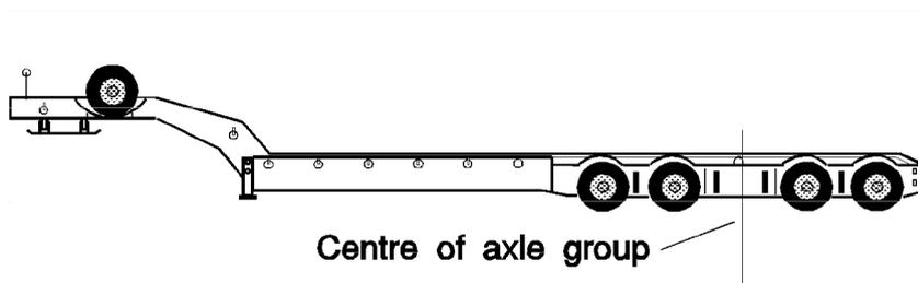
**Centre of a typical quad-axle group with an equal number of tyres**
