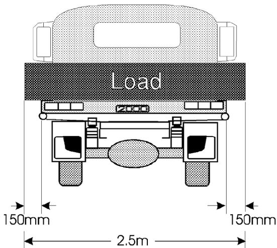
**A vehicle loaded to width limits mentioned in section 7 with maximum side projection of load permitted under this section.**
