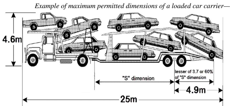
In the above example, the 'S' dimension is the distance between the trailer's front articulation point and its rear overhang line.
