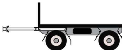
**drawbar** means a part of a trailer, other than a semitrailer, connecting the trailer body to a coupling for towing purposes.
