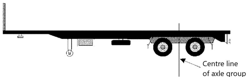
*Example of the centre line of a tandem axle group fitted with a different number of tyres on each axle—*
