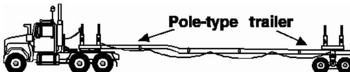
*Examples of loads generally capable of supporting themselves like beams between supports—*
