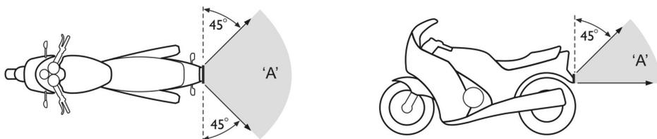
**Number plates must be clearly visible from 20 metres at all points within arcs 'A'**
