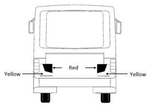
Example of an alternative patter for rear marking plates—
