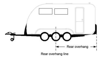
Example of the rear overhang and rear overhang line for a semitrailer-
