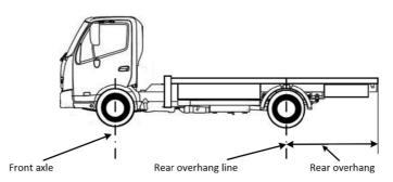
Example of the rear overhang and rear overhang line for a motor vehicle—
