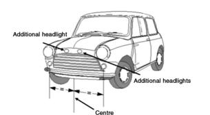
Example of the position of additional headlights fitted to a vehicle-
