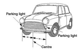
Example of the position of a pair of parking lights fitted to a motor vehicle with 4 wheels—
