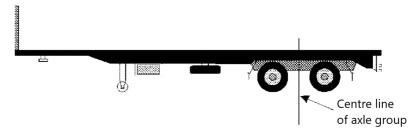
*Example of the centre line of a tandem axle group fitted with a different number of tyres on each axle—*
