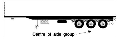
Centre of a typical tri-axle group with an equal number of tyres
