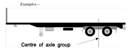
Centre of a typical tandem axle group fitted with an equal number of tyres on each axle
