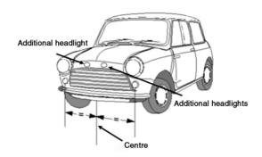
Example of the position of additional headlights fitted to a vehicle—
