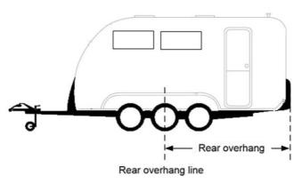
*Example of the rear overhang and rear overhang line for a vehicle with a tri-axle group at the rear—*
