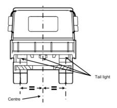
(4) Tail lights fitted to a vehicle in accordance with this division may also serve as rear clearance lights if the tail lights are fitted to the vehicle in accordance with section 89(3).
