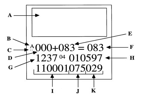
*A* is details written by the operator of the system's camera, when a film magazine is inserted, that are superimposed on each image on the film as it is taken.
