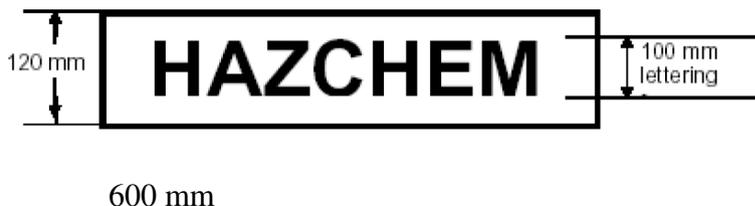
**Figure 13.1 Form and dimensions of outer warning placard**
