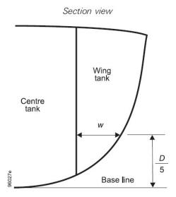
w must be at least 2 metres along the entire length of the tank for the tank to be used in the calculation of  $PA_c$
