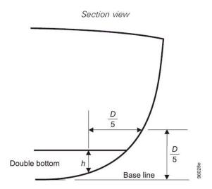
h must be at least 2 metres or  $\frac{B}{15}$ , whichever is less, along the entire length of the tank for the tank to be used in the calculation of  $PA_s$
