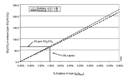
Figure  $1-SO_2/CO_2$  versus % sulphur in fuel
