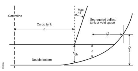
If h is less than 2 metres or  $\frac{B}{15}$ , whichever is less, anywhere along the tank length, but  $h_{\rm db}$  is at least 2 metres or  $\frac{B}{15}$ , whichever is less, along the entire tank length within the width of 2b, then:
