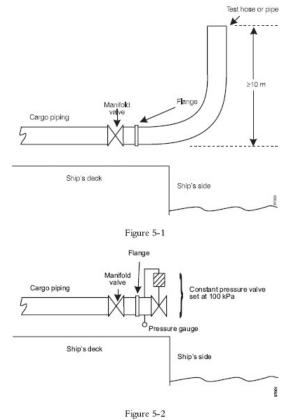
The above figures illustrate test arrangements that would provide a backpressure of not less than 100 kPa at the cargo tank's unloading manifold.
