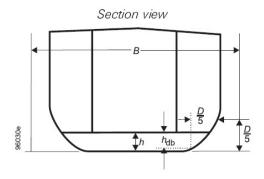
If  $h_{db}$  is at least 2 metres or  $\frac{B}{15}$ , whichever is less, along entire tank length,
