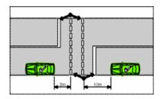
Measurement of distance-marked foot crossing
