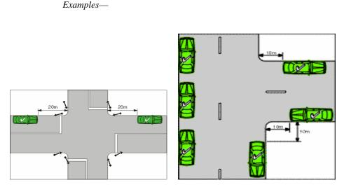
Example 1 Measurement of distance—intersection with traffic lights
