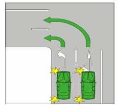
Starting a left turn on a multi-lane road with traffic lane arrows as required or permitted under section 92
