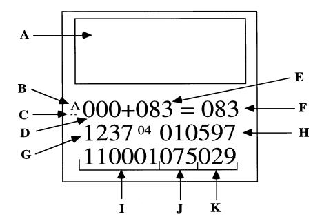
A is details written by the speed camera's operator, when a film magazine is inserted, that are superimposed on each image on the film as it is taken.
