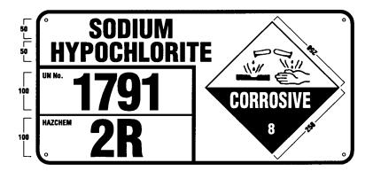
figure 4—example of completed emergency information sign for single class of hazardous substance
